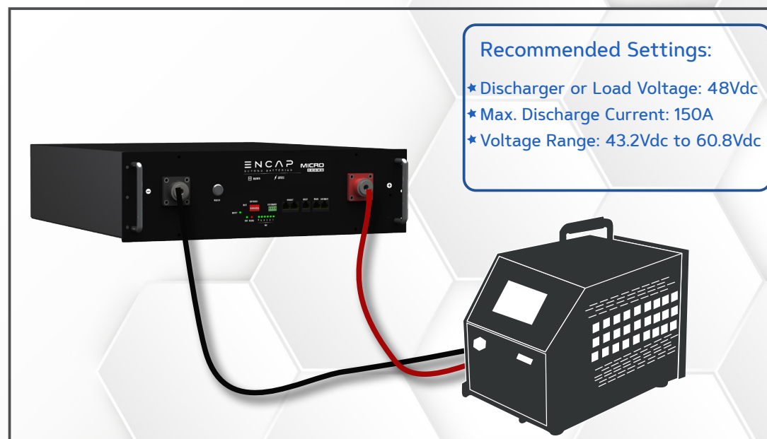
Figure 12: Discharging Module from discharger
